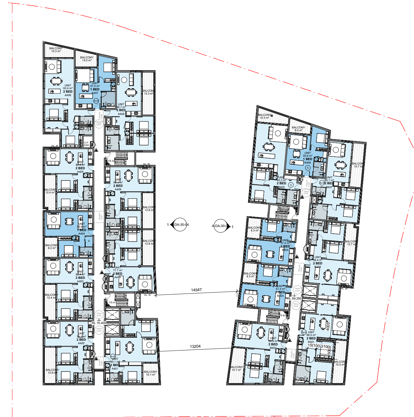
Typical level 4 tower A and tower B
